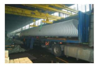
In comparison to the classical installation of corrugated steel structures mentioned above the client must only lift the structure in one step from the forwarding vehicle into the end position and saves himself thus precious time on the construction site.
