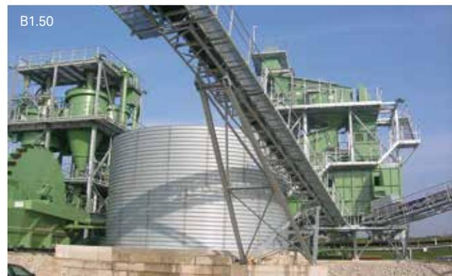
The **Hamco Multi-Plate** construction method enables the manufacturing of **water tanks** with a diameter of max. 30,54 m and a height of max. 6,10 m as well. Those water tanks are similar to the silos for bulk material, but during the assembly an elastic band is laid in all vertical and horizontal seams. Furthermore steel beam as well as foundations are not necessary.
